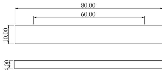
Flexural testing specimen; ASTM D790 (ISO 178,GB/T 9341)
