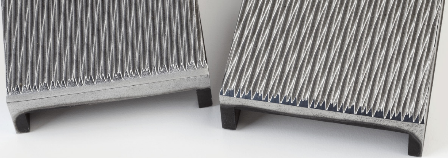
Industrial die, printed using LPBF
